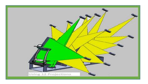
A 3D-image can be reconstructed from projections of an object. The number of projection affects the reconstruction quality. A larger number projections will lead to better reconstruction quality. On the other hand, less projection number can reduce the radiation dose, save time and speed up the baggage inspection. You can see the result of reconstruction algorithm on our data in below.
